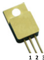
TO – 257 (Isolated Base-plate Hermetic Package)
