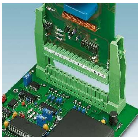
4. ICV 2,5 versions and MSTB 2,5 headers to create primary/secondary PCB connections. Here, FLRP lateral guide rails are used to stabilize the secondary PCB.
