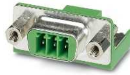
Shielded POWER SUBCON header for wall thicknesses of up to 4.5 mm, 4-40 UNC fastening thread, with leading medium PE contact
