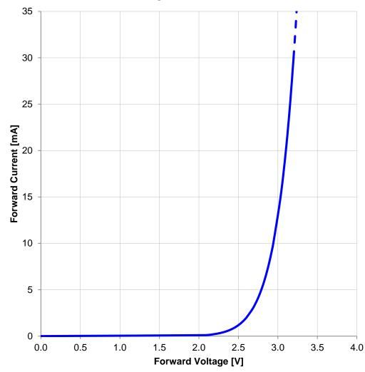
CHECKED GENERAL TOLERANCE PROJECTION METHOD CREATED Würth Elektronik eiSos GmbH & Co. KG EMC & Inductive Solutions KaS PLD DIN ISO 2768-1m Max-Eyth-Str. 1 74638 Waldenburg **WL-SMCW SMD Mono-color Chip** Tel. +49 (0) 79 42 945 - 0 **LED Waterclear** ORDER CODE www.we-online.com 150060BS75000 eiSos@we-online.com DATE (YYYY-MM-DD) BUSINESS UNIT REVISION STATUS PAGE 002.008 Valid 3/8 0603 2017-12-01 **WÜRTH ELEKTRONİK**
